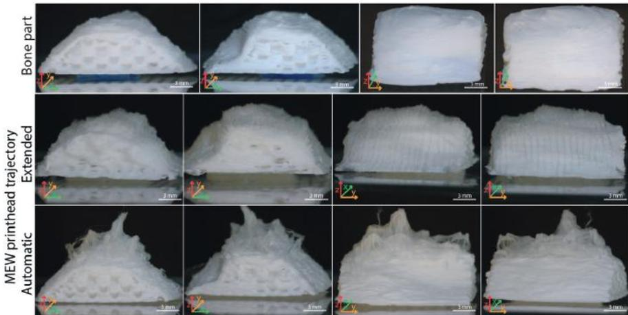
**Figure S3. Macroscopic images from all sides of the bone part and the resurfaced implants with the manually extended and fully automatic code.**
