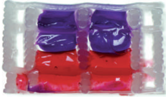
Figure 3. Layering of the hydrogels results in specific confinement of the printed hydrogels. The layers are shown using differently stained hydrogels ( A ) and hydrogels containing fluorescent microspheres (size 15 \mu\text{m} , B ). Scale bar represents 2 mm.
