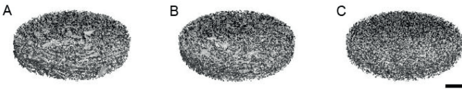
Figure 1: Micro-CT images of the different scaffolds 100:0 (a), 50:50 (b), 0:100 (c). These images illustrate the differences in particle size between the groups. Scale bar represents 1 millimeter.
